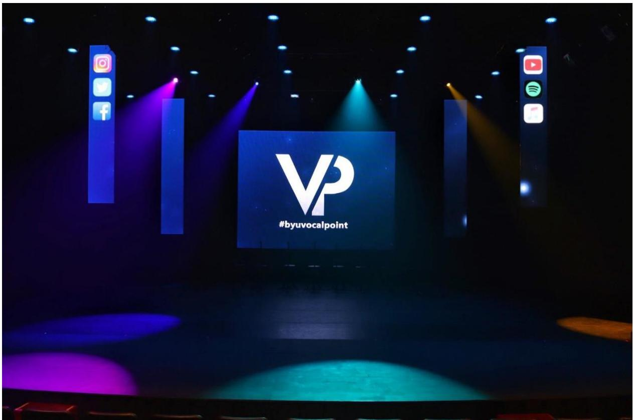
*A normal configuration of the LED screens, with a main screen in center, and two “pillars” on each side. This configuration requires the use of 3 depths of batten or truss.*
